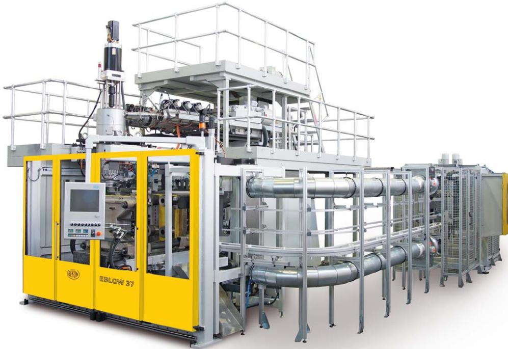
By intelligently combining electric and hydraulic drive technology, BEKUM makes the most of the benefits of each technology, offering customers the ideal conditions for high-capacity production of blow moulded articles, especially canisters from 10 l to 35 l.
