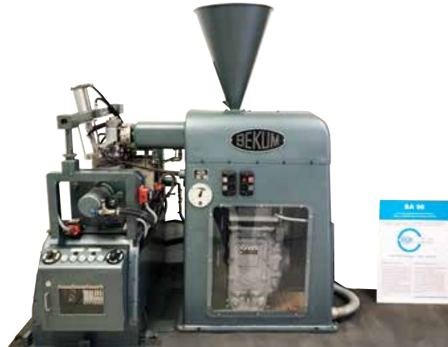
BA 90 – the worldwide first blow moulding machine with the patented „inside-neck dimensioning system“
