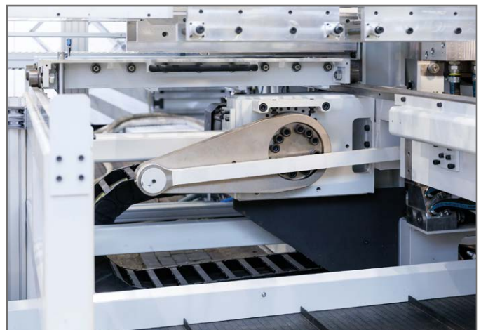
Electric crank for carriage movement
