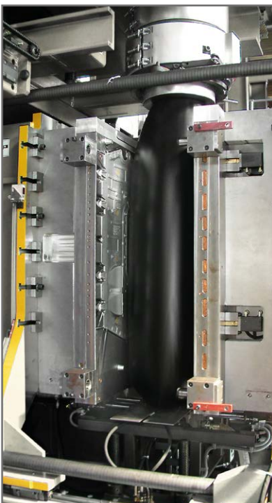
Large clamping unit for long technical parts
