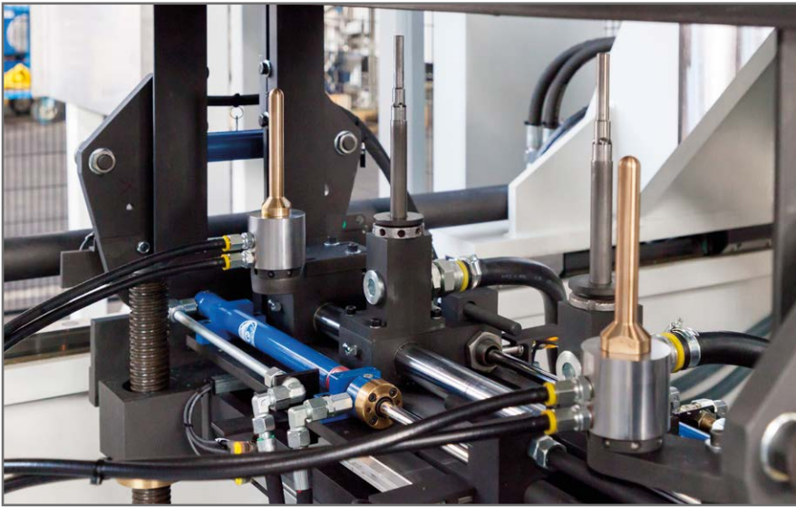
Bottom calibration with parison spreading device
