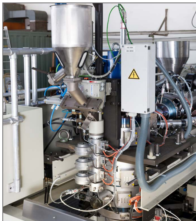
BA 34.2D Tri-Extrusion of canister with view strip
